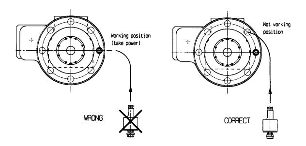
At the end of the equipment, all the DIN 69880 seats, which are not occupied, by static or rotating toolholder, must be closed with plugs DIN 69880 (Z2) and with its locking screws
