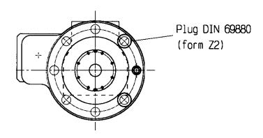
It's compulsory to avoid that chips, go through the VDI or its screw seat. Before remove the toolholders from the disk, clean the area with air. If these rules are not followed, it coul be damaged the correct functioning of the turret
