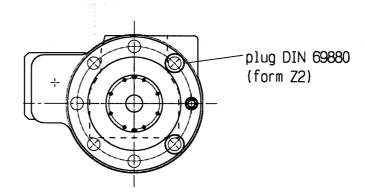
It's complusory to avoid that chips, go through the VDI or it's screws seats. Before remove the toolholders from the disk, clean the area with air if these rules are not followed, it could be damaged the correct functioning of the turret
