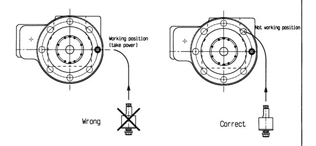
At the end of the equipment, all the DIN 69880 seats, witch are not occupied, by fixed or rotating toolholders, must be closed with plugs DIN 69880 (Z2) and with its looking screws
